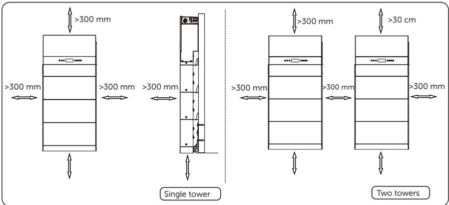
Figure 4-7 Clearance requirement
