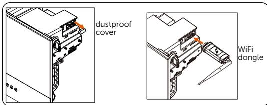
Figure 7-66 Pulling out the dustproof cover and plugging in the WiFi dongle
