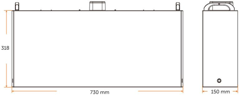
Figure 2-6 Battery module
