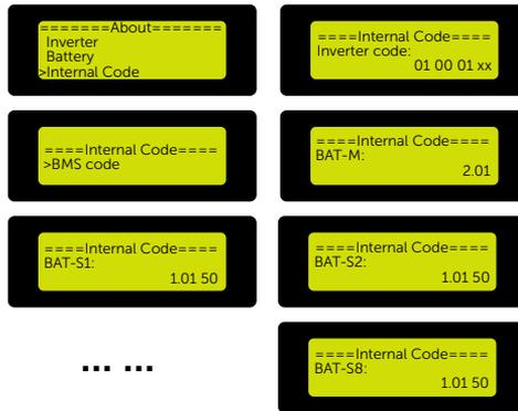
Figure 9-104 Displaying the internal code information
