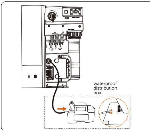
Figure 7-60 Meter connection
