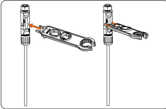
Figure 12-5 Inserting the tool into the PV connector
