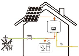
In case of power failure, the system will supply EPS loads through PV and battery. ((The battery must be installed. And the EPS loads must be less than the minimum of the following two values: the sum of the maximum battery discharge power and the maximum PV output power, or the overload limit power of the inverter.)
