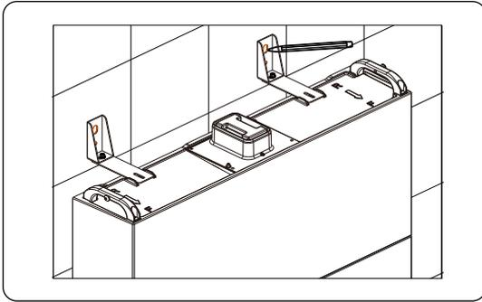
Figure 6-40 Marking the position of BMS
