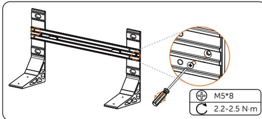
Figure 6-31 Attaching base support and transverse plate
