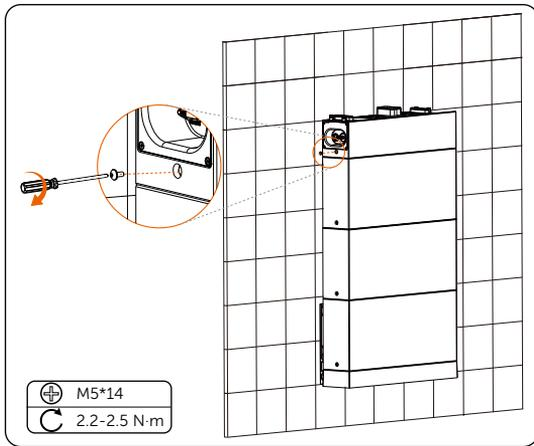
Figure 6-47 Tightening M5 screws
