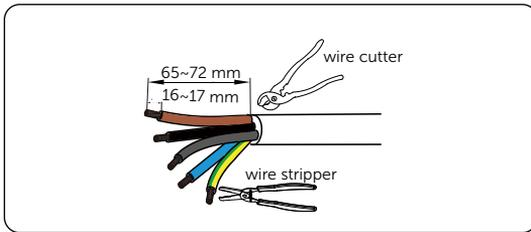
Figure 7-15 Stripping the Grid and EPS cables
