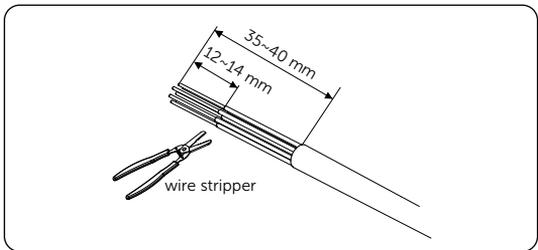
Figure 7-48 Stripping cables
