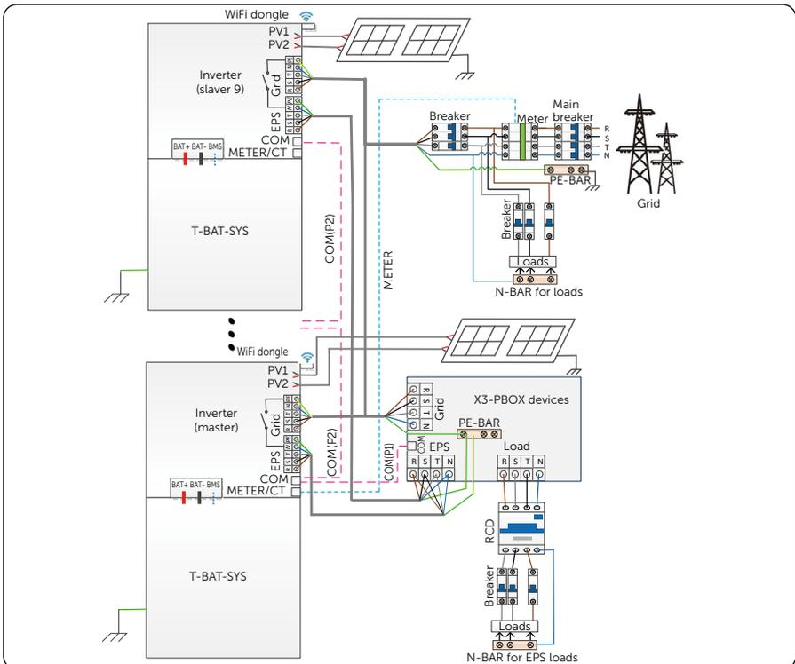
Figure 7-37 System diagram with SolaX X3-PBOX device
