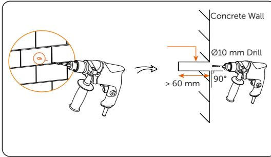
Figure 6-9 Drilling holes
