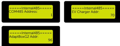
Figure 9-97 Setting the address of the external device
