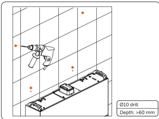
Figure 6-19 Drilling holes
