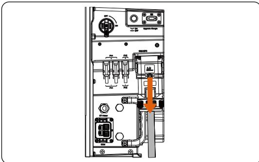
Figure 12-10 Disconnecting the Grid&EPS cable
