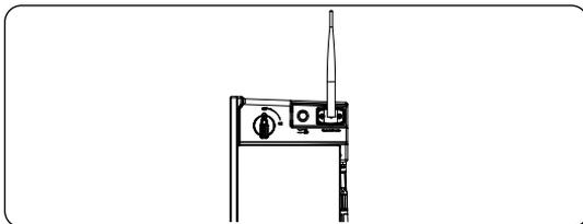
Figure 7-67 Well connected WiFi dongle
