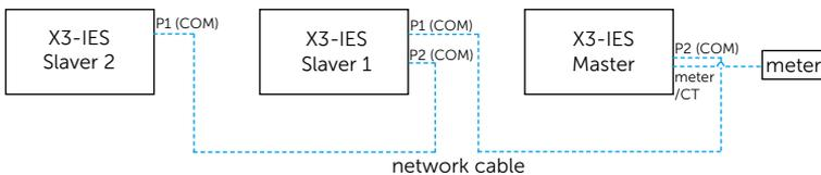
Figure 7-40 Parallel connection without SolaX X3-PBOX device
