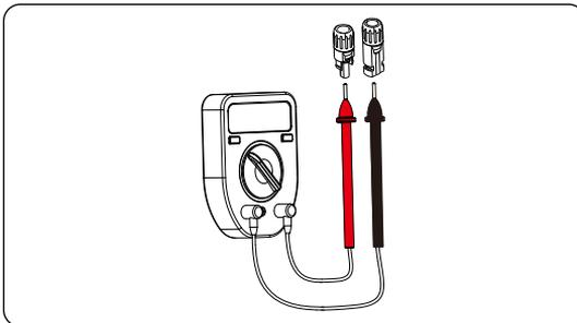
Figure 12-7 Measuring the voltage of PV connectors
