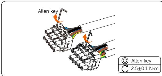
Figure 7-20 Locking wires in the AC connector
