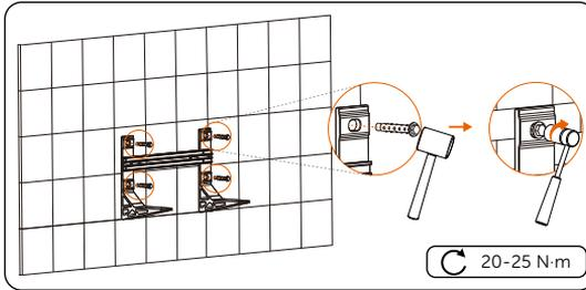
Figure 6-34 Tightening expansion screws
