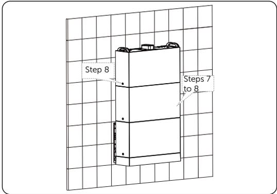
Figure 6-38 Placing battery modules
