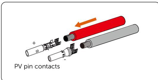
Figure 7-29 Inserting PV pin contacts into PV cables
