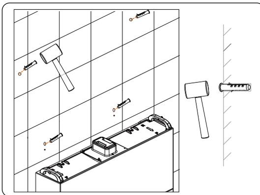
Figure 6-44 Knocking expansion tubes into the wall
