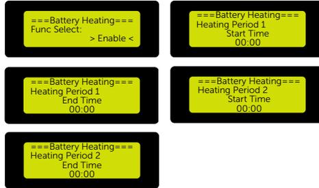
Figure 9-91 Enabling battery heating and setting working periods
