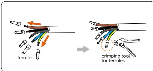
Figure 7-16 Crimping the Grid and EPS cables
