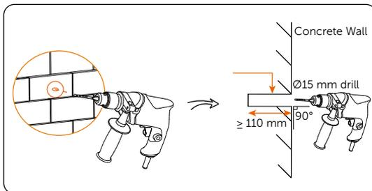
Figure 6-33 Drilling holes
