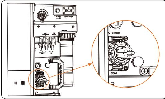
Figure 7-44 Well connected COM port
