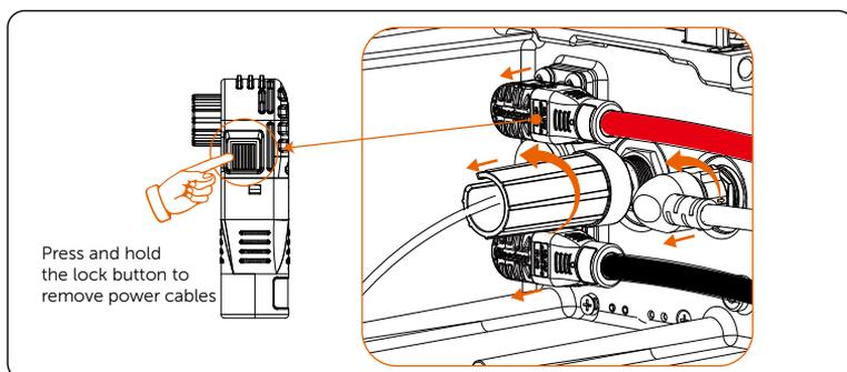
Figure 12-14 Disconnecting battery connectors
