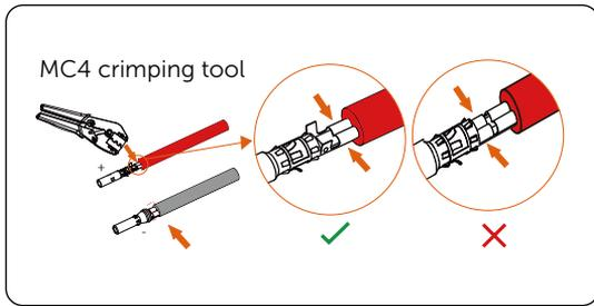
Figure 7-30 Crimping cables with PV pin contacts
