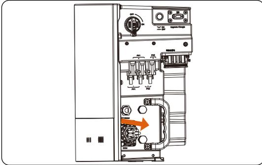
Figure 12-11 Disconnecting the communication connector
