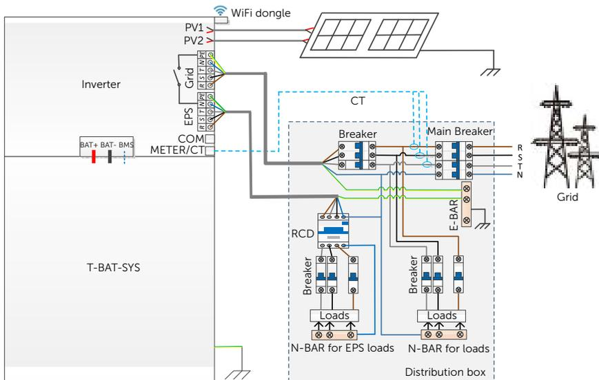
Figure 2-21 System diagram for Australia
