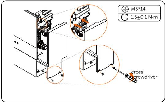
Figure 7-61 Locking the cable shielding board
