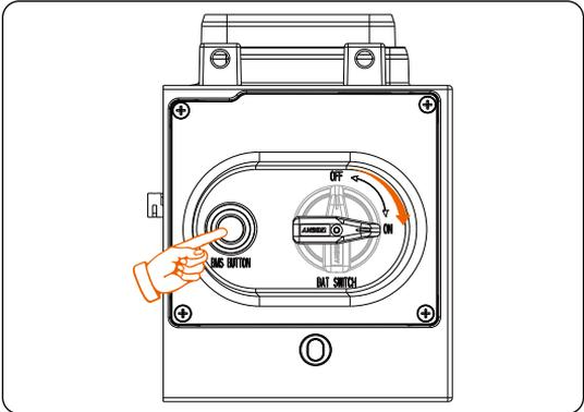
Figure 8-3 Turning on the battery
