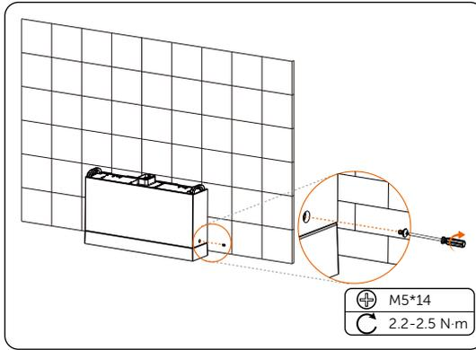
Figure 6-13 Tightening screws
