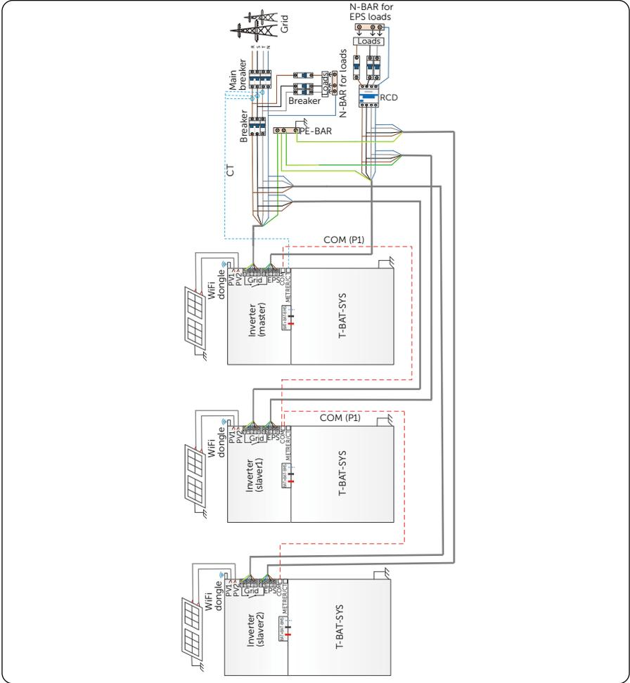
Figure 7-38 System diagram without SolaX X3-PBOX device
