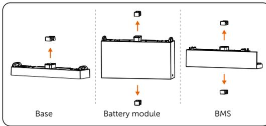
Figure 6-30 Removing dust covers
