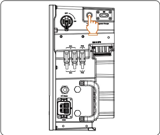
Figure 8-4 Pressing the inverter button
