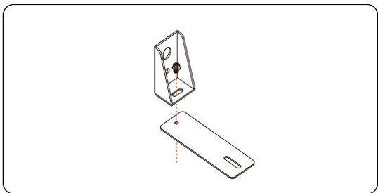
Figure 6-39 Attaching two brackets
