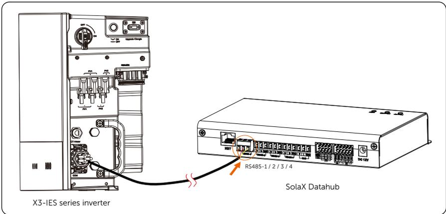
Figure 7-41 Inverter connected with a SolaX datahub
