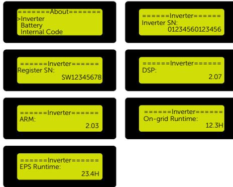
Figure 9-102 Displaying the inverter information
