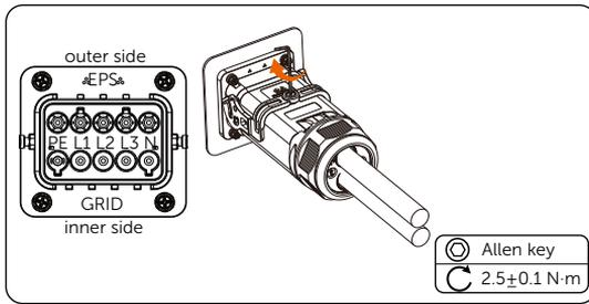
Figure 7-25 Tightening the lock on the AC connector
