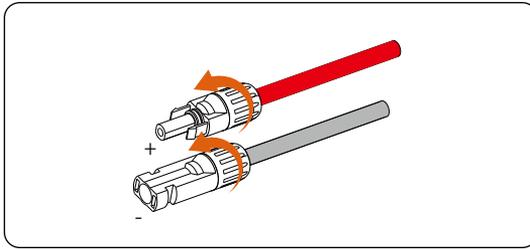
Figure 7-33 Tightening swivel nuts of PV connectors
