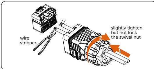
Figure 7-46 Stripping cables
