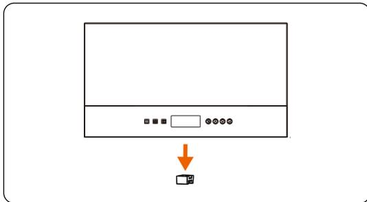
Figure 6-48 Removing the dustproof cover
