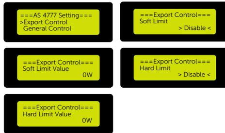
Figure 9-73 Setting export control in AS4777 setting interface
