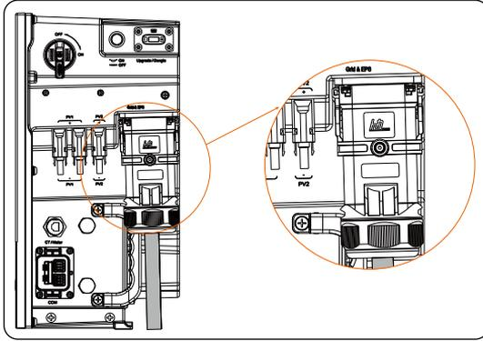
Figure 7-14 Well connected Grid & EPS cables
