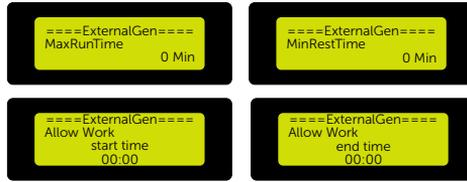
Figure 9-82 Setting MaxRunTime, MinRestTime, allow working period
