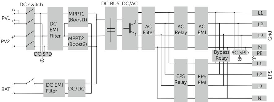
Figure 2-19 Circuit Diagram
