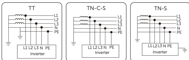
Figure 2-2 Supported power grid
