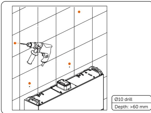
Figure 6-43 Drilling holes
