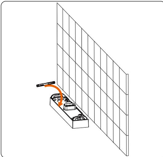
Figure 6-4 Determining whether the base is level
