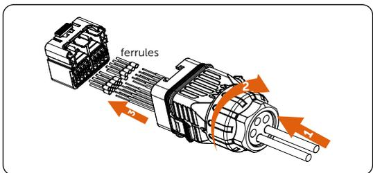
Figure 7-49 Inserting wires into ferrules
