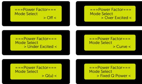
Figure 9-55 Selecting a mode in power factor
