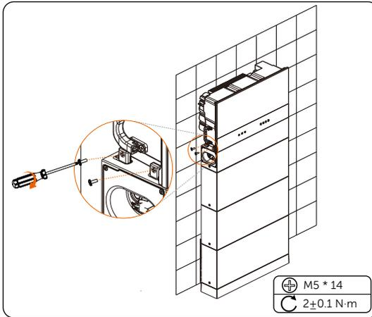
Figure 6-26 Locking the inverter with the BMS
