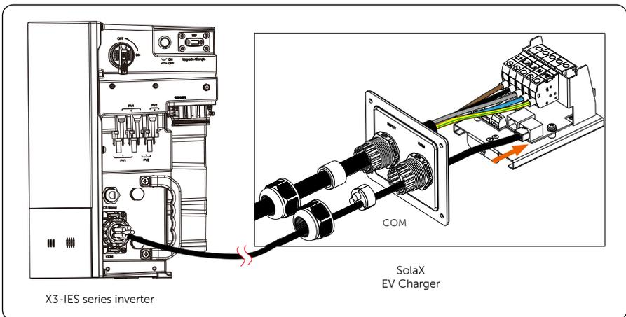
Figure 7-42 Inverter connected with a SolaX EV Charger
