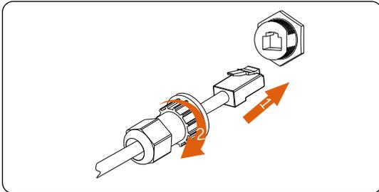
Figure 7-58 Connecting cable to the Meter/CT port
