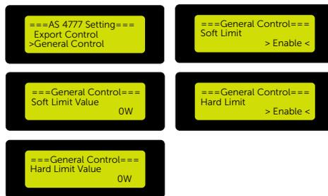
Figure 9-74 Setting general control in AS4777 setting interface
