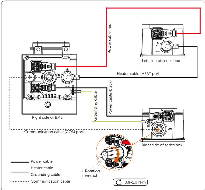
Figure 7-9 Connecting cables
