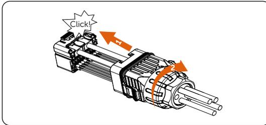
Figure 7-51 Inserting the terminal block into the connector
