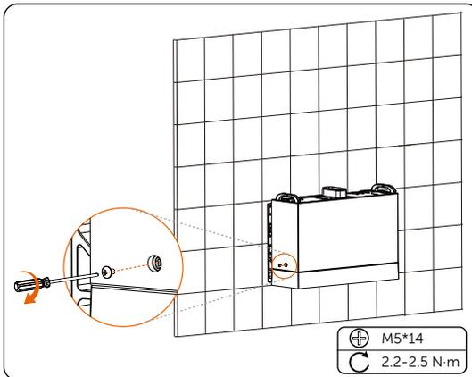
Figure 6-37 Tightening screws
