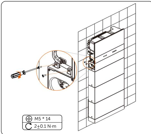
Figure 6-50 Locking the inverter with the BMS
