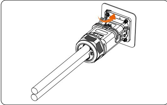
Figure 12-8 Loosening the AC connector
