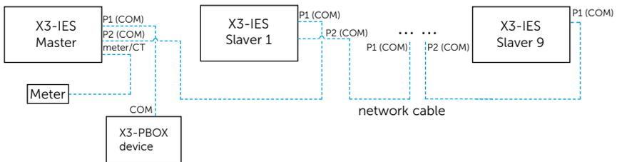
Figure 7-39 Parallel connection with SolaX X3-PBOX device
