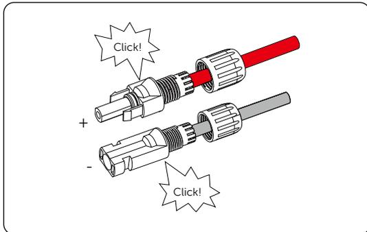
Figure 7-32 Securing PV cables
