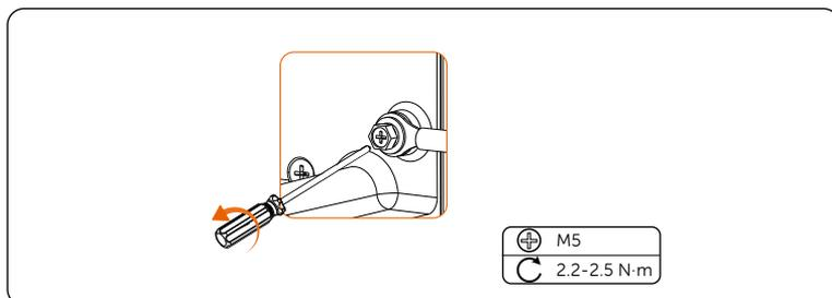
Figure 12-15 Disconnecting grounding cable
