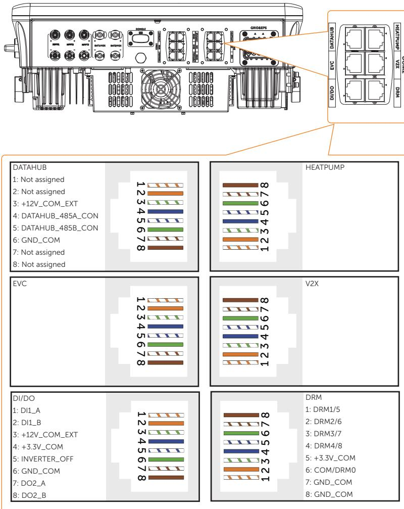
\* The pin assignment for sub-terminals HEATPUMP, EVC, and V2X is not shown in details, because these sub-terminals are suitable for the standard RJ45 plug.
