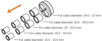
According to the outside diameter of the cable, take out the corresponding sealing plug from the cable support sleeve.
