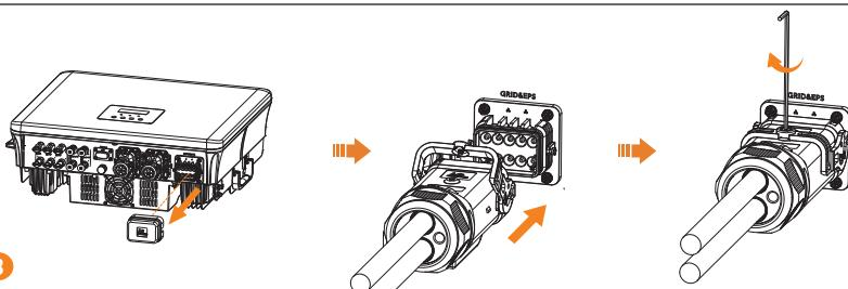
\*Before the inverter is powered on, make sure that the AC connector has been properly connected to the Grid side of the Grid & EPS terminal. Otherwise, it will cause a high-voltage electrical shock, resulting in serious personal injury or even death.
