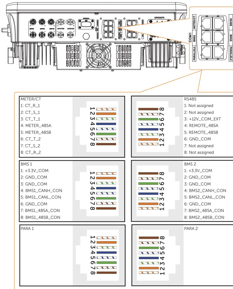
\*The pin assignment for sub-terminals PARA 1 and PARA 2 is not shown in details, because these sub-terminals are suitable for the standard RJ45 plug.
